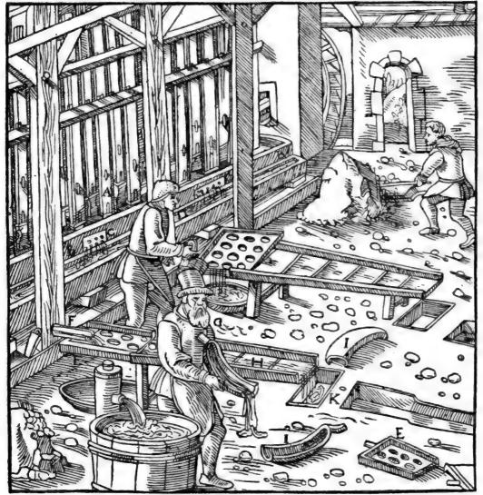
A—Stamps. B—Mortar. C—Plates full of holes. D—Transverse launder. E—Planks full of cup-like depressions. F—Spout. G—Bowl into which the concentrates fall. H—Canvas strake. I—Bowls shaped like a small boat. K—Settling-pit under the canvas strake.
